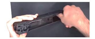
Depress extractor with thumb, then pull retaining pin out of the top of the bolt.
