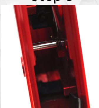
Insert the upgraded sear spring in the orientation show with the short leg facing inwards and the long leg visible in the slot in the grip. Partially insert the sear pin from left-to-right to retain the spring.
