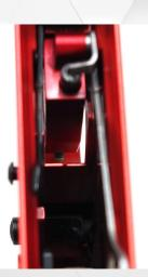
Reinstall the trigger spring and detent and lower the disconnector bar over the detent.
