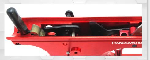
Insert the safety plate and hook the front edge over the tip of the sear. You may need to pull the sear forward into alignment. Hold the safety plate in place with one hand and start the safety lever and shaft into the hole and through the safety plate to retain the safety plate.
