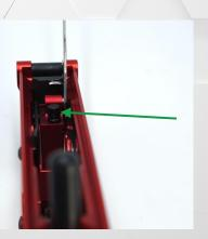
Remove the hammer, hammer bushing, magazine disconnect components, and safety plate. The magazine disconnect components and hammer will not be re-installed.
