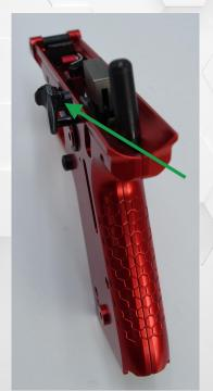
Grip the safety lever and pull it away from the frame while wiggling up and down.
