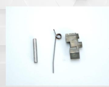
With your small punch, drive out the sear pin. Remove the sear and sear spring. The factory sear and sear spring will not be reinstalled.
