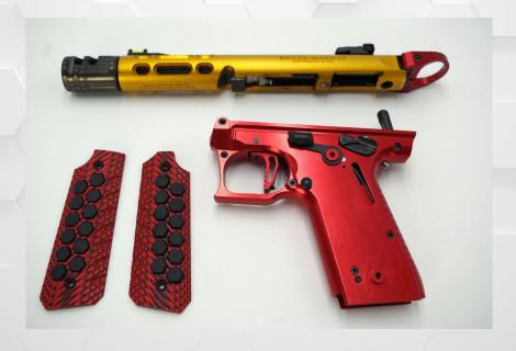
Detach the upper from the lower according to your pistol's manual and remove the grips.
