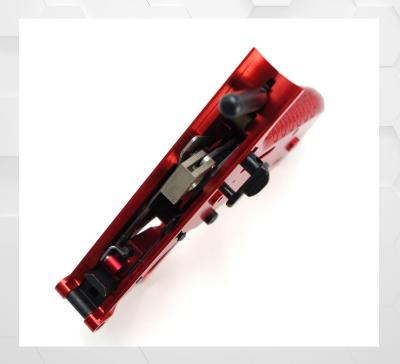
Pressing down on the connector bar, insert the hammer assembly into the pistol, making sure that the hammer strut is pressing onto the mainspring plunger and the hammer bushing is inside the square cut-out of the connector bar. Press the safety shaft through the hammer assembly, and connector bar, but not all the way through.
