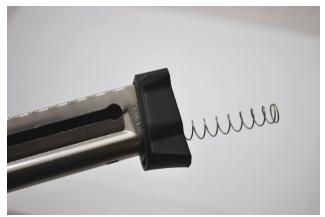
7. Screw in the three screws into the appropriate spaces to secure the halves together and your +5 magazine bumper is now complete!
