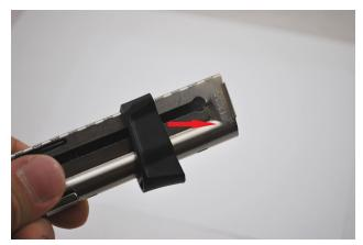
6. Feed the new spring into the magazine and then carefully depress the spring with the lower half of the bumper until it snugs onto the upper half of the bumper.
