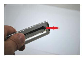
5. Slide the upper half of the bumper over the top of the magazine and bring it down over the button hole.
