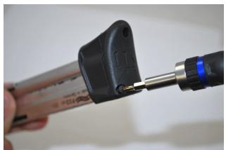
8. If you experience feed issues when utilizing the magazine: We include a small black shim that can be used to place under the spring to assist with the last round feeding. If you have difficulty with the last round feeding utilize the included shim and place it into the bottom of the basepad under the spring and re-install.
