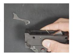
Install the trigger housing back into the receiver.
