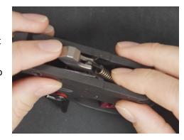
Orient the ejector as shown and insert the remaining pin in its hole in the left side of the housing - through the bolt release plate, and through the ejector. Rotate the hammer spring forward so the bent leg sits in the notch on the bolt release plate, then press the straight leg down so that it is held under the pin as you push it the rest of the way into the housing.
