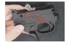
Punch out the pin that holds the disconnector in the trigger. Put the disconnector into the new trigger shoe as shown and replace the pin.
