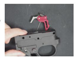
Put the loop of the bolt lock spring around the right side of the bushing on the hammer. Orient the hammer as shown. The spring leg with the slight bend it should be to the front. Put the hammer into the housing and put the largest of the pins through the frame and hammer. The hammer and spring should be able to move freely.
