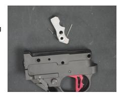
Put the wide end of the hammer spring assembly into the hole at the rear of the trigger housing. The slot in the retaining clip should be in the 12 o'clock position. Insert the thin end of the hammer strut into the slot on the back of the hammer. Pull the hammer back until it locks in the cocked position. The wire spring should still be able to move freely.
