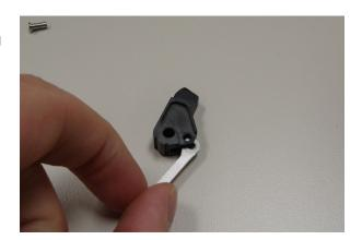
2. Insert the hammer strut pin into the hole through the hammer and the strut. It must be inserted from the right side of the hammer, where there is a recessed area around the hole. If inserted from the left side, it will not function correctly.
