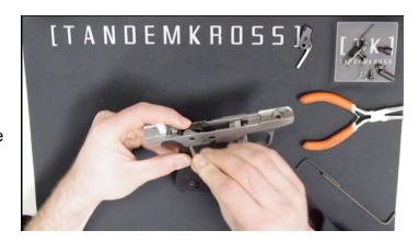
7. Replace the spring in front of the safety. To avoid scratching the frame of your gun, use a brass punch to compress the spring into it's space.
