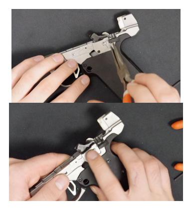
5. Lift the factory hammer out of the gun and set it aside, then place the Thunder Hammer in the gun where the factory hammer was. The flat face of the hammer should be facing the front of the gun, and the strut should be toward the back of the gun and pointing down towards the main spring.
