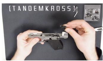
6. Apply gentle downward and forward pressure to the hammer so that the holes through the frame, safety, hammer, and trigger bar all line up, then re-insert the hammer pin from the right side. Tip: Rotate the top of the hammer toward the front of the gun to assist with hole alignment.
