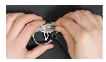
9. Cock the hammer. If the hammer refuses to pull back, it means the hammer strut is misaligned with the main spring. Push the hammer all the way forward, then pull it back, and it should align itself correctly. Test the functionality of the safety and trigger. If both work as expected, cock the hammer again and replace the barrel. **Note: the barrel will not reattach is the hammer is not cocked.**
