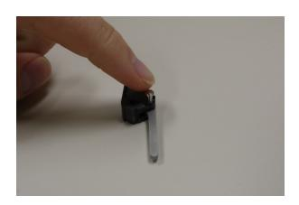
3. If the strut pin is inserted correctly, the flat surface of its head will be flush with the highest surfaces on the side of the hammer. If inserted incorrectly, the flat surface of the strut pin's head will be the highest on the side of the hammer. If your reassembled hammer look like the picture below left, re-insert the pin on the other side of the hammer so it looks like the picture below right.
