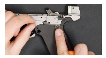
8. Replace the bolt stop lever, the left grip plate, the magazine release and spring, and the right side grip plate.
