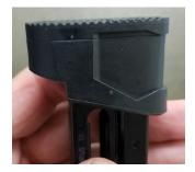
9. Insert an allen wrench or similar tool in the track of the magazine near the bottom and hook onto the spring. Pull toward the top of the magazine and slowly release to make sure the spring has not buckled in the bottom of the bumper.
