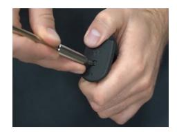
2. Slowly slide the factory base plate off of the magazine being careful to not allow the spring and spring plate escape.
