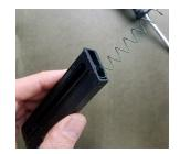
6. Slide the top half of the new Wingman bumper over the magazine in the orientation shown.
