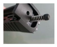
4. Slide the striker housing sub-assembly out of the rear of the slide. It is easier if you can keep the housing halves, striker, striker block and spring together. If it falls apart it is not hard to put everything back together. Take extra care not to lose the spring. The spring is very small and can be very difficult to find (speaking from personal experience).
