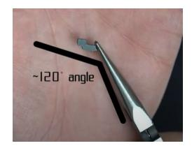
9. Install the extractor detent and spring. Notice that when the detent is installed in the proper orientation that approximately three coils of the compression spring are exposed (shown to the right). The step in the detent needs to align with the step in the rear of the extractor. If the detent is not installed properly there will be approximately five coils exposed.
