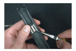
8. With extractor oriented in the needle nose plier as shown right. Insert extractor into breech block. Rotate extractor into position.
