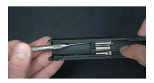
7. Using needle nose pliers manipulate the extractor out the front of the breech block. Shaking or tapping the slide may help coerce the extractor out of the breech block.
