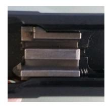
10. Install striker block sub-assembly. The exploded view is from the Tx-22 manual.
