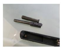
2. Depress retainer slide cap with allen wrench. The cover plate can start to slide with spring and detent compressed.
