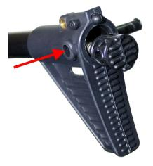
2. The entire buttstock will now need to be removed by removing the stock pin even further than the stopping point groove machined into it. This is done by lining up the detent (green arrow) with the center cut out in the pin (red arrow) and then rotating the pin counter-clockwise such that the detent no longer rides in the groove of the stock pin. We recommend to slowly pull the pin out a bit more so that the stock can be slid off but still have the pin retain the detent if possible.
