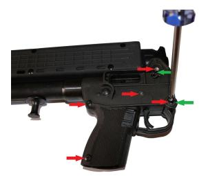
3. Repeat steps 1 and 2 on the other side of the firearm as it is symmetrical. Remember to replace the washers under the two screws closest to the muzzle (green arrows).
