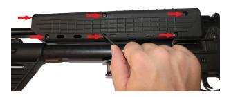
Troubleshooting: If one of the deep screws on the forend fails to come out with a screwdriver or magnet you will need to remove all the screws on that side of the forend and push it out from the inside. Replace the forend side plastic, align the forend, and secure with hex screws.
