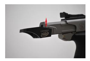
Step 3: Install and tighten the included 5-40 7/8" socket cap screw. Do not overtighten the screw. The charging handle grips tightly to the bolt. Some blue loctite is recommended to keep it from working loose.
