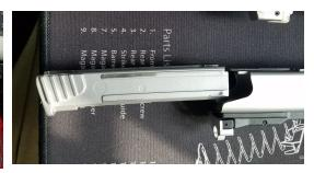
2. With the bolt positioned as shown, push end of original factory guide rod through the slot to remove it. Position the new captured spring with brass washer toward the bolt face and the brass cap towards the rear of the bolt. Compress the spring by pressing on brass cap (about 1/8") and slide into the slot of the bolt.
