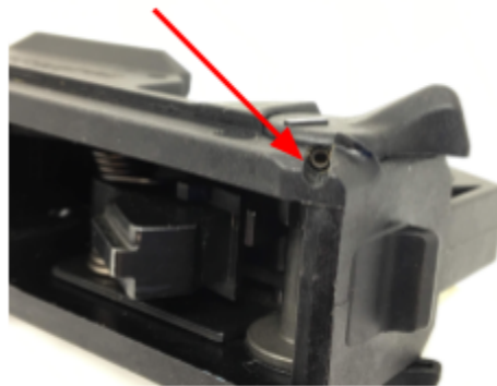
REMOVE RIGHT-SIDE SCREW IN SAFETY SELECTOR
