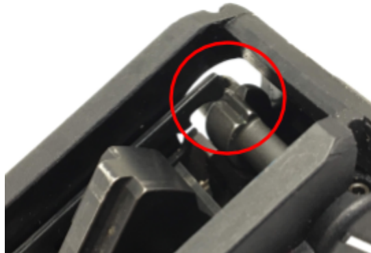
ALIGN DETENT FINGER WITH DETENT GROOVE
