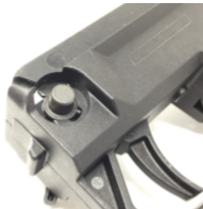
PUSH ON EXPOSED SAFETY PLUG
