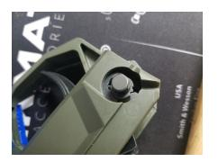
4. Align the line on the safety delete with the line on the safety switch. Install the "Kross Out" Safety Delete using the original set screw. Re-install the trigger sub-assembly.
