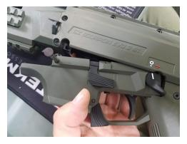
3. Push out magazine release roll pin with punch. Be careful to not lose the compression spring.
