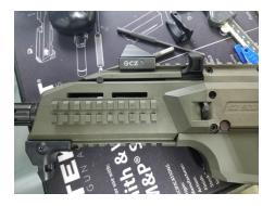
2. Identify the takedown captured pin. Push from the right side to the left side of firearm. Remove the trigger sub-assembly
