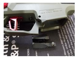
4. Install the new magazine release and stock compression spring in trigger sub-assembly. Compress the spring to align the hole in the magazine release with the hole in frame. Install the roll pin.
