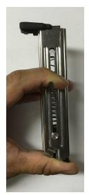
3. Slide the follower to the bottom of the magazine, line it up with the hole and remove it from the magazine. Leave the follower inside the magazine.
