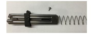
4. Slide the upper half of the bumper over the top of the magazine and bring it down over the button hole. Replace the follower button in the follower. Feed the spring back into the magazine and then carefully depress the spring with the lower half of the bumper until it snugs onto the upper half of the bumper.
