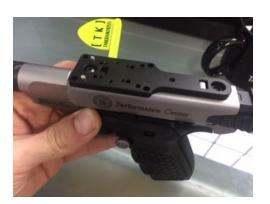
Install the dowel pins in locations specified in table for the forward mounting position. Pins may have a small amount of resistance sliding in holes.
