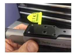
If you are installing a Trijicon RMR or Holosun HS507C, use the included cone head set screws in either holes 1 and 2 (for forward mounting), or 3 and 4 (for rearward mounting). Insert these screws from the underside of the mount so that the point of the set screw protrudes beyond the upper surface of the plate to fully engages the counterbores in the bottom of the sight. The screws are adjusted properly when the sight has no side to side or front to back play.
