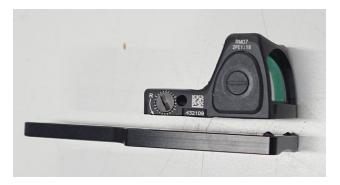
Place the sight on the mount in proper alignment with pins. Verify that sight is flush with the mount. Check to be sure that the correct length screws are being used. Install and firmly tighten the mounting screws using medium strength thread locking compound. Do not exceed 8 inch-pounds of torque when tightening flat head #4 screws.
