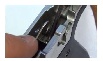
9. With the sear rotated forward, insert the safety and then the hammer back into the gun. The tail of the hammer must drop into the pocket behind the sear toward the rear of the gun. The hammer is easiest to install with it rotated slightly toward the front of the gun pressing it down onto the sear. Align the holes and insert the pin from the RIGHT to LEFT
