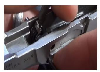
8. Begin reinstalling the trigger disconnect bar over the top of the sear. Rotate the sear toward the front of the gun, and hook the opening in the trigger disconnect bar over the sear.
