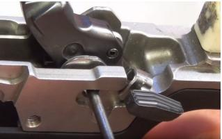
Lift up on the trigger disconnect bar. You
