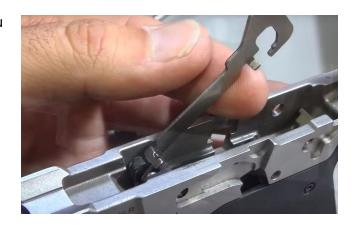
7. With the disconnect bar lifted up, press the trigger pin out from LEFT to RIGHT and it will slide out easily. Lift the trigger, trigger spring and trigger disconnect bar out of the top of the gun. Set the trigger and trigger spring aside. You will need the trigger pin later.
