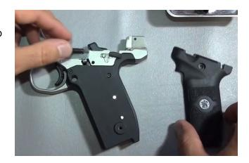
4. Make sure that the hammer is not cocked. If you still have the magazine disconnect installed you may need to insert an empty magazine into the grip to be able to pull the trigger to release the hammer.
