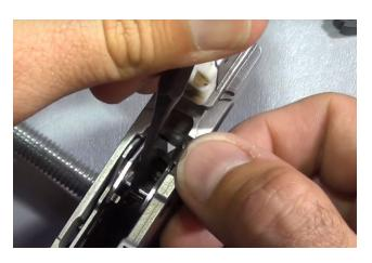
capturing the Safety first and then the hammer and finally the left side of the gun. Reinstall the pin retaining clip
