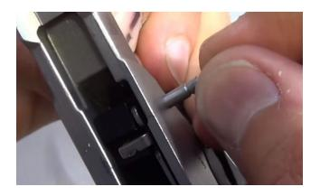
14. Slide the included bushing down the LEFT side of the trigger and over the hole for the trigger pin. Finish pushing the trigger pin through the bushing.
