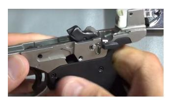
5. With the hammer in the uncocked position remove the retaining clip that holds the hammer pin in place. Using a pick or similar small tool will help removing the retaining clip. The pin will push out from LEFT to RIGHT and will allow for the safety and hammer to come out of the gun.
