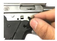
4. Start threading the included screw through the paddle button. Once it starts coming out the other end, screw it to the "Titan". Adjust button position as preferred.
