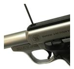
2. Slide the sight rail to the right and up off of your SW22 Victory. If the sight rail does not slide easily, wiggle to loosen it.
