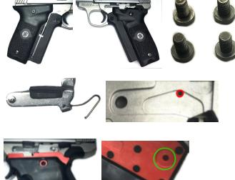
4. Screw in the grip screws from earlier by starting with the top left screw. Press the grip forward as you tighten the top left screw to ensure proper fit under the safety. Next tighten the bottom left, then top right and finally bottom right.
