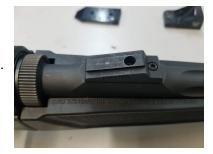
Remove the two torx head screws from sight base and then remove the sight base.
