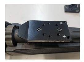
If required, install dowel pins in the locations specified in the table for the forward mounting position. Pins may have a small amount of resistance when inserting into the holes.
