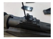
Remove the rear peep sight by sliding it off of the dovetail slot.
