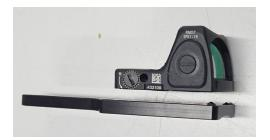
Place the sight on the mount in proper alignment with the pins. Verify that the sight is flush with the mount. Check that the correct length screws are being used. Install and firmly tighten screws using medium strength thread locking compound. Do not exceed 8 inch-pounds of torque when tightening flat head #4 screws.
