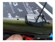
Remove rear sight assembly by pushing it out of dovetail slot from the left side of the firearm using a drift or sight pushing tool being careful not to damage the firearm. Sometimes the rear sight can be very tight in the dovetail and it may warrant a visit to your local gunsmith for removal.
