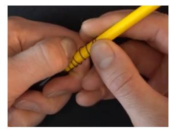
4. Replace the plunger on the end of the spring, compressing the spring all the way down into the body of the magazine so that the plunger is flush with the end.
