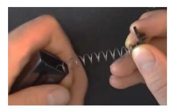
3. Insert the new "Green Spring" into the magazine and carefully compress it, one coil at a time, into the body of the magazine. A pencil or similar tool through the middle of the spring can be used to help guide it in.
