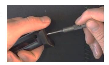
Carefully slide the base pad off the end of the magazine and remove the spring and plunger. Set the stock spring aside. You will not need it again.
