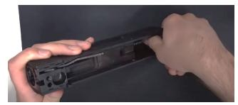
7. Replace trigger housing. Align holes in trigger housing with holes in the receiver and replace the two dowel pins.
