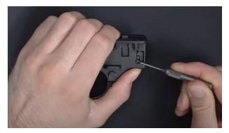
5. Insert "Bolt Keeper" in place of original bolt lock and replace retaining pin.
