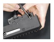
4. Press up on the bolt lock, then use the punch to push out its retaining pin.
