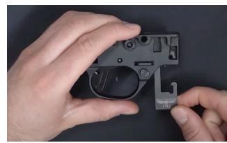
6. Replace trigger housing. Align holes in trigger housing with holes in the receiver and replace the two dowel pins.
