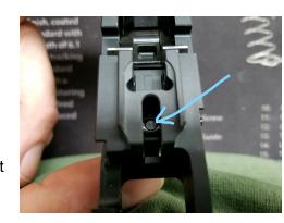
It is NOT necessary to remove the safety rocker, however if it falls out during the installation it is VERY IMPORTANT to re-installed in the proper orientation per Ruger Instructions and picture right.
