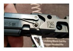
While holding trigger bar assembly together, drop bolt release spring into frame insert as shown.
