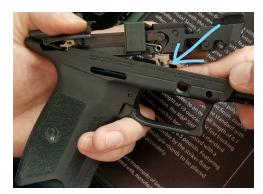
Slowly seat the front end of the frame insert. The retaining clip will be pushed off the frame insert as it seats into the grip.
