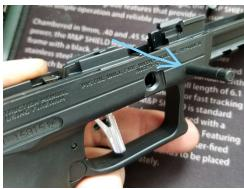
Install take down lever clocked as shown.
