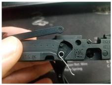
Wind leg of spring counter clockwise and secure under trigger bar. Notice groove in bottom of trigger bar.
