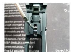
Insert trigger bar into fire control under the tab on the sear.
