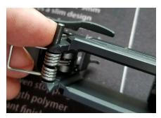
Install barrel pin.
