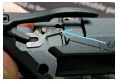
11. With the trigger pivot pin removed, the trigger spring and pivot can be removed from the trigger. The trigger then slides out the bottom of the frame.
