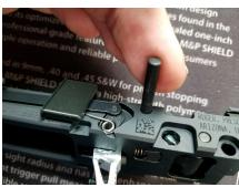
Verify the hammer is standing straight up. This will reduce the force on the hammer spring. Drop the back end of the frame insert into the grip frame first. The grip frame should be pushing the hammer spring down and forward as you are mating the two parts.
