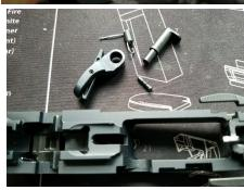
12. Install the pre-travel and overtravel screws. Set the overtravel as shown right. Set the pre-travel with the head of the screw flush with the face of the trigger as shown. If the pre-travel screw is not flush the pivot pin hole will not be accessible to install the pivot pin.
