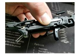
6. Release the trigger spring from the trigger bar (if that has not already released itself).
