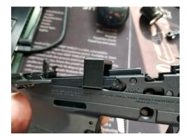
Install frame insert pin.
