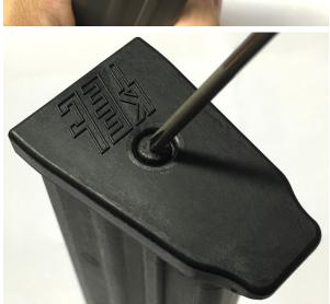
3. While the plunger is depressed, grip the base plate with your hand and slide it off the magazine base. Be mindful of the spring and keep it depressed with your thumb if able.
