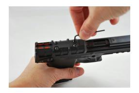
2. Align the screw holes, with the slope of the new TANDEMKROSS PMR-30 rail toward the *rear* of the PMR-30, with the slope of the built-in sight on the slide cover.
