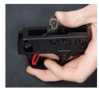
11. Rotate hammer towards the front of the gun. Install main spring. The washer that captures the spring is inserted into the counterbore in the trigger housing. There is a window in the side of the trigger housing that allows access for fully seating spring into housing. The spring strut fits into the slot in the back of the hammer. Rotate hammer towards rear of the gun to compress and capture main spring in trigger housing. Turn on safety so that the trigger doesn't get inadvertently pulled.
