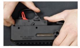
10. This is a good time to verify that the bolt release componentshave remained in the trigger housing. Verify that the bolt release plate/button, bolt release pin, and bolt release spring are present and accounted as shown. If these parts have fallen out, install spring into counter bore, compress spring with bolt release button/plate, install dowel pin, release button.
