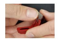
8. Take the nylon tipped screw out of the hardware bag and screw it metal end first into the hole on the rear face of the trigger. This will be your overtravel adjustment screw. You can use the included allen wrench to adjust it to your liking once the install is done.
