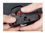
10. Insert hammer into trigger housing, with slot for main spring strut towards the rear of the gun. Align hammer with thru hole in trigger housing. The hammer will be compressing sear slightly when in the proper position. Install hammer pin.
