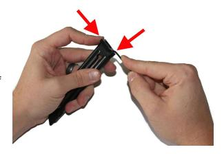
4. If unable to keep the spring depressed, you should be able to push it back in with your thumb and index finger. Firmly pinch the plunger with your thumb and index finger, and push it down in small increments. Be sure to use your other hand to keep the spring from jumping out.
