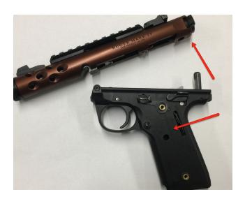
2. Uncock the pistol. Place an unloaded magazine into the pistol, put the safety on fire and pull the trigger. Alternatively you can lift the magazine safety with a tool and pull the trigger.
