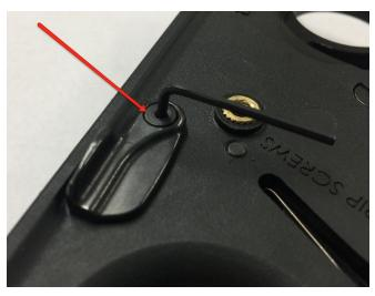
4. To facilitate an easy installation insert a small allen wrench or similar under the lower edge of the sear to keep it from rotating back when the hammer is removed.
