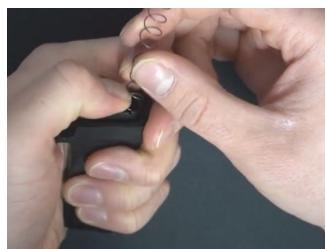
Place the bottom half of the "Wingman" bumper over the end of the spring and compress the spring until the two bumper halves are in contact.
