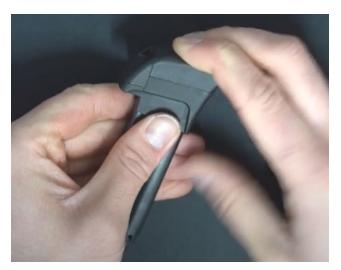
6. While holding the two halves of the bumper in place, screw the two screws into the screw holes on the bottom and top halves of the "Wingman".
