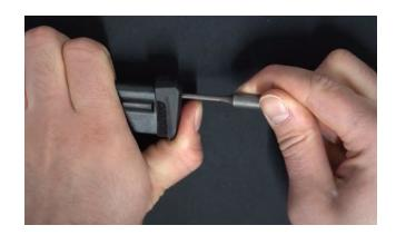
Carefully slide the bumper off the end of the magazine and remove the spring and plunger. Set these aside. You will not need them again.
