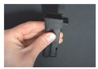
4. Insert the new "Green Spring" into the magazine and carefully compress it, one coil at a time, into the body of the magazine. A pencil or similar tool through the middle of the spring can be used to help guide it in.
