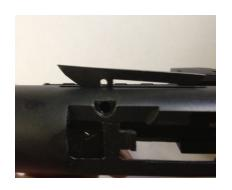
5. If your LCI is not fitting into the slot: On some models of 22/45 LITE the barrel is twisted in the aluminum shroud and it comes down into the LCI slot area where the flag portion of the LCI replacement needs to be seated into the slot. Looking into the slot if you see a portion of the barrel coming down into the slot and the LCI does not fit you will need to sand the edge of the LCI.
