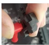
10. Carefully assemble the two sides of the lower together. Align the mainspring pin first. Keep the left side of gun down to help keep the feed ramp from disengaging the bolt lever. Press the trigger disconnect bar down past the safety window in frame.
