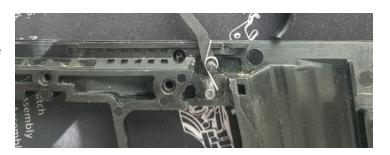
7. Install the pre-travel screw and overtravel screws. Both screws are installed with hex towards the face of the trigger.
