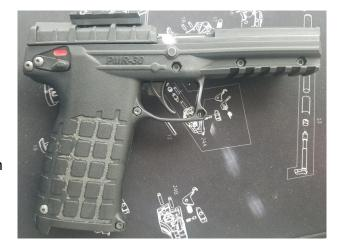
3. Remove all screws from the right side of the firearm. Take note that the button head cap screws on magazine release and safety lever are longer than the rearmost screw. It will require two allen wrenches to remove the magazine release screw.
