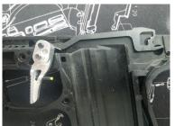
9. Install the feed ramp and torsion spring into the left side of the frame. The free end of the spring must be wound counterclockwise about 180 degrees to insert it into bolt release lever. Utilize the TK tool to aid in install.
