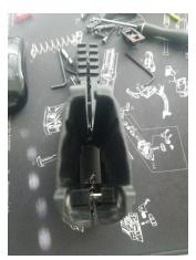
6. Raise disconnect bar to release force on torsion spring and remove stock trigger. Notice that free end of torsion spring rests behind the lower dowel pin.
