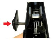
4. Install the Accelerator cross pin from LEFT to RIGHT. Be sure the tension spring for the slide stop plate (highlighted in red) is captured underneath the cross pin.
