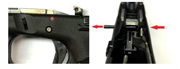
2. Using a punch or similar tool, remove the trigger pin (highlighted in red) from LEFT to RIGHT.
