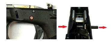
3. Be sure the through holes are aligned before installing the Accelerator from LEFT to Right.
