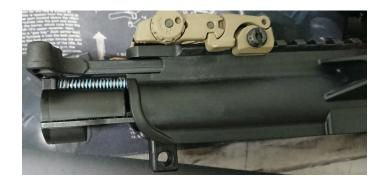
4. Separate the bolt assembly from the charging handle.
