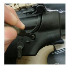
2. With the disassembly pin pushed out, open the gun by pushing down on the front handguard.
