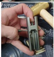
7. With the firing pin removed, remove the spring from the original firing pin, and put it onto the new firing pin. Remember that the wider part of the spring goes to the back of the firing pin, and the thinner part goes to the front.
