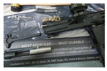
5. Next, take the bolt assembly, and pull back the recoil spring to remove the spring rod. The spring rod has cuts in it so that you can pull it out easily. Pull it straight up from the plastic retainer and then remove the spring rod and spring.
