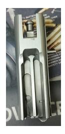
9. Now, we can put the guide rod back onto the bolt. The correct orientation of the plastic rear section is with the notch for the spring rod facing up. Then you will place the spring rod with the spring on it back through the hole in the bolt, and compress the spring so that you can put it back into the spring rod holder.
