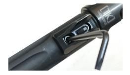
Apply medium strength thread locker (such as blue Loctite) to one of the T10 Torx screws and place it in the hole of the new fiber optic sight.
