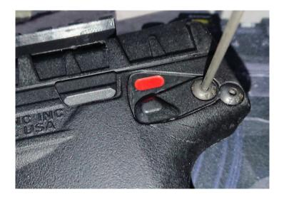
3. Remove the old safety lever, keeping in mind where the slots of the safety mechanism are.
