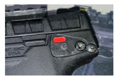
4. Place the "Cornerstone" thumb ledge safety into the safety mechanism, ensuring that the slot on the thumb ledge aligns with the key on the safety mechanism.
