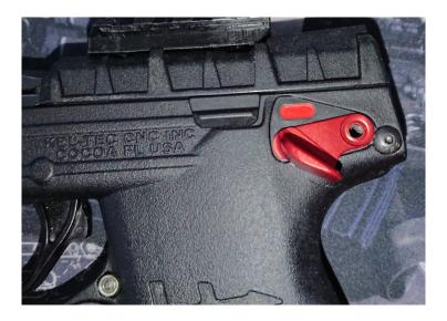
5. Replace the retaining screw, turning the allen wrench clockwise until the safety switch moves to the up position. To ensure that the safety is tightened, switch it between safe and fire, and check for any movement. If there is none, you have completed the installation correctly!
