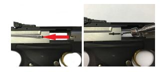
Step 3: Pressing down on the plunger with the back of the extractor slide the new extractor into the slot in the side of the bolt. There should be an audible click as the extractor locks into place. The extractor should have good movement as it pivots in the slot.
