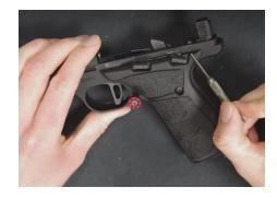
7. Turn the gun over and remove the punch, allowing the sear spring to fall out.
