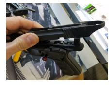
6. Remove sear spring pin with pin punch. Leave the punch in the gun to retain the spring.
