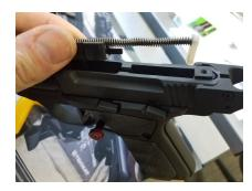
4. Lift up and remove the slide.
