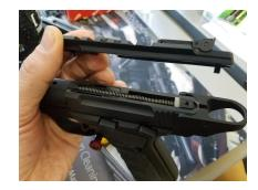
3. Remove the firing pin housing, recoil spring and buffer.
