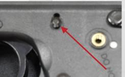
The underside of the "Bolt Keeper" has a keyhole-shaped cutout. This will fit over the stud on the internal bolt stop (part numbers 9&10 in the owner's manual).
