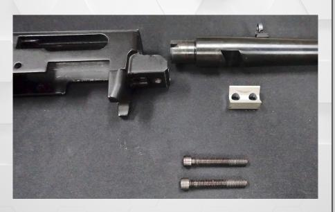
V-block attachment screws. The screws will be reused. The factory V-block will not be reinstalled
