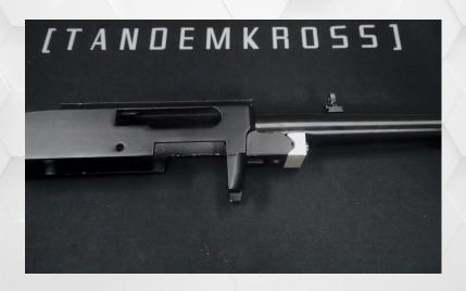
Remove your barreled receiver from the stock. Detach the trigger housing.
