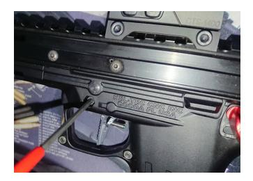
2. From the right hand side push the takedown pin out slightly so that the lip of the pin will be accessible. Use a punch if necessary.
