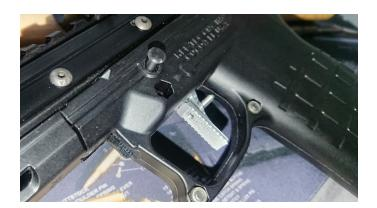
3. Slide the Accelerator onto the takedown pin and position it so that you can put the extended allen screw through the frame of the gun. Then tighten the allen screw.
