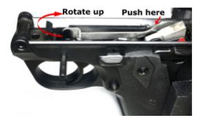
5. With a dental pick or similar tool gently lift UP on the retaining spring while pressing on the magazine release. **Be aware, the spring is under pressure.**
