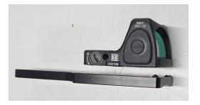
Place the sight on the mount in proper alignment with pins. Verify that sight is flush with the mount. Check that the correct length screws are being used. Install and firmly tighten screws using medium strength thread locking compound. Do not exceed 8 inch-pounds of torque when tightening flat head #4 screws.
