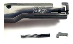
Step 4: Release the plunger with the new extractor in place and the pressure from the spring will self align the new extractor with a snap.
