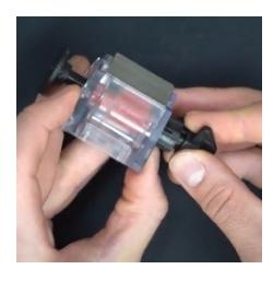
9. Insert the shoulder bolt, making sure it goes through the center of the spring coils, and tighten with the allen key.
