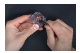
2. Remove the back side of the magazine housing and pop the stock nut out of it. Set the stock nut aside, you won't be needing it again. Leave the other components of the magazine in place.
