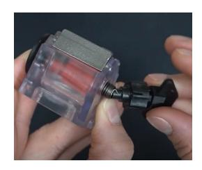
8. Turn the Hex Nut 2 full turns with the wing nut holder. Once the spring tension is high enough the hex nut will start to pull into the housing. Press the hex nut into the housing firmly. \
