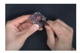
2. Insert the spring into the new rotor and use the needle nose pliers to maneuver the short bottom leg of the spring into the hole in the side of the rotor.
