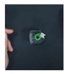
5. Snap on the back side of the magazine housing. This will line up with the small stud on the feed lip and the center of the rotor. The hex cutout is facing out.
