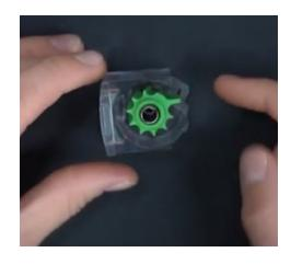
4. Install the Feed Ramp. The LARGER alignment stud goes toward the BOTTOM, small stud on top. Looking close at the metal feed lip you will see one of the corners is cut off. This corner faces the inside of the housing.
