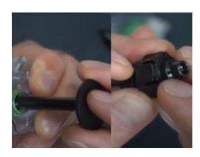
7. Locate the hole in the bottom of the Hex Nut and align it to the end of the spring. Remove the spring lifter.
