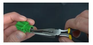
3. Place the rotor into the housing. The spring faces UP. Large tab facing out of the slot.
