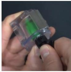
9. Insert the shoulder bolt, making sure it goes through the center of the spring coils, and tighten with the allen key.
