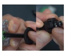
7. Locate the hole in the bottom of the Hex Nut and align it to the end of the "Green Spring". Remove the spring lifter.
