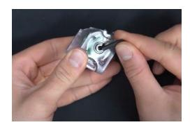
2. Insert the new "Green Spring" into the new rotor and use the needle nose pliers to maneuver the short bottom leg of the spring into the hole in the side of the rotor.
