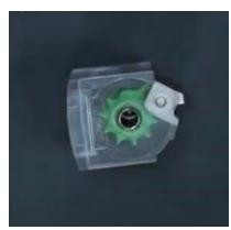
6. Insert the spring lifter into the bottom of the TANDEMKROSS 10/22 Double Kross Housing. This will push up the "Green Spring" from the inside. Using the Nut holder, insert the Hex Nut into the holder.
