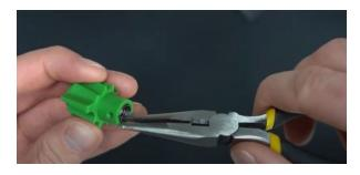
3. Place the rotor into the housing. The spring faces UP. Large tab facing out of the slot.
