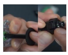
7. Locate the hole in the bottom of the Hex Nut and align it to the end of the spring. Remove the spring lifter.
