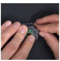
6. Insert the spring lifter into the bottom of the TANDEMKROSS 10/22 Double Kross Housing. This will push up the spring from the inside. Using the Nut holder, insert the Hex Nut into the holder.
