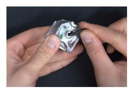
3. Place the rotor into the housing. The spring faces UP. Large tab facing out of the slot.
