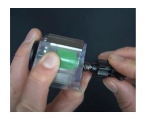
8. Turn the Hex Nut 2 full turns with the wing nut holder. Once the spring tension is high enough the hex nut will start to pull into the housing. Press the hex nut into the housing firmly. \
