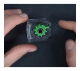
4. Do not re-install stock feed lip. Instead, install the TANDEMKROSS Feed Lip. The LARGER alignment stud goes toward the BOTTOM, small stud on top. Looking close at the metal feed lip you will see one of the corners is cut off. This corner faces the inside of the housing.
